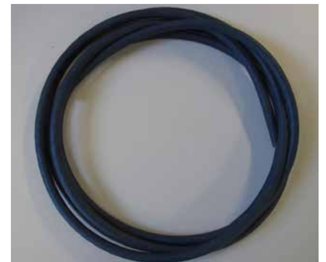
Result chainflex® TPE jacket: Cable after the 520,000 strokes test
