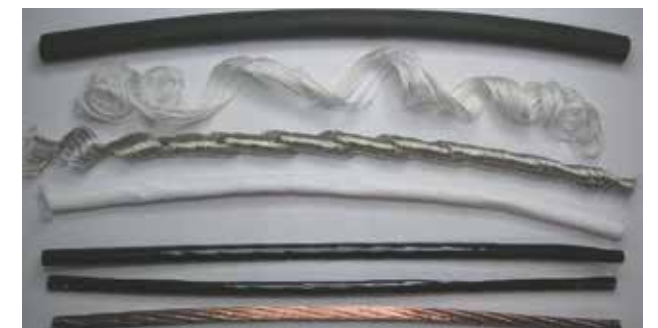
Picture 2: The CFROBOT shows absolutely no damage after more than 3 million movements
