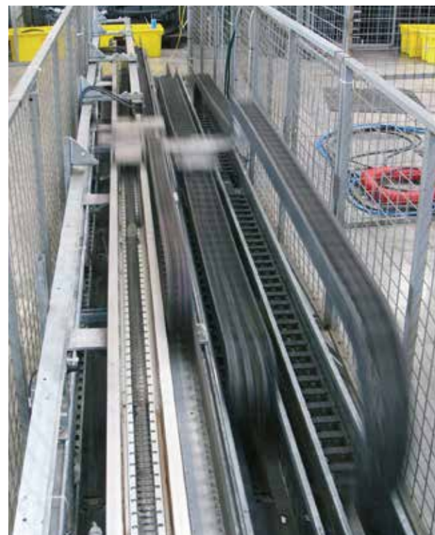
Picture 1: Gliding e-chain® application as the basis of the test
