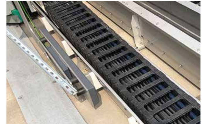
P4.1 e-chain® with EC.PP in the igus® outdoor test
