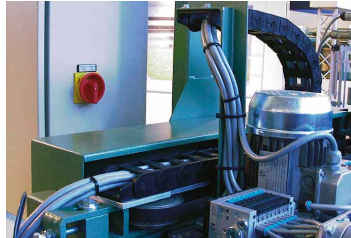
chainflex® CF140.UL in a feeder application. e-chain®: easychain®
