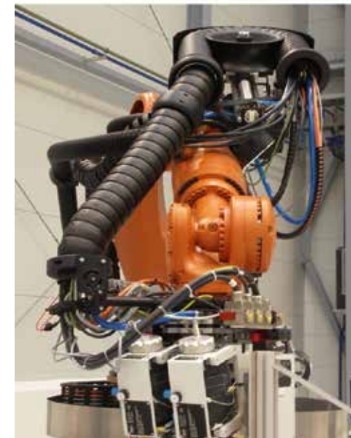
igus® chainflex® cables in a triflex® R multi-dimensionally moving energy supply system for 6-axis robots
