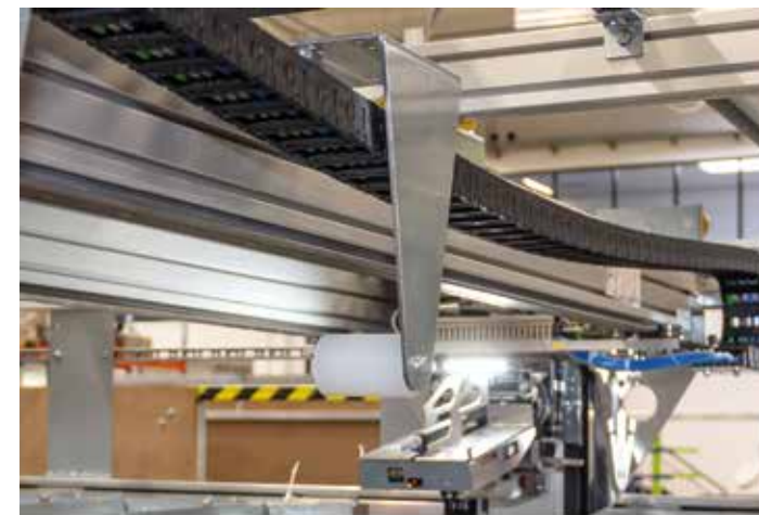
chainflex® cables (e.g. CF211) and igus® e-chains® (E065 series) in a pharmacy picking systems
