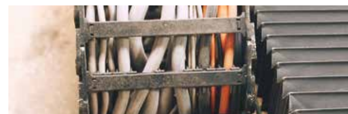
Corkscrewing: an effect of improper cable and hose placement in an e-chain®
