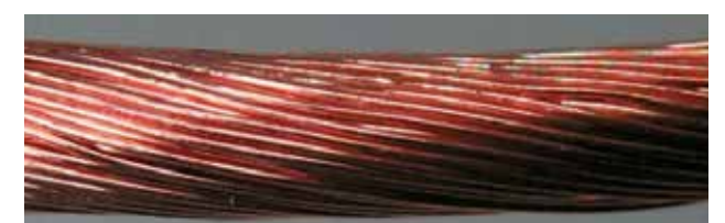
A close-up of the completely intact copper conductor. The inspection performed over the entire length shows that the conductor is still completely intact and does not have any individual strand wire breakages.
