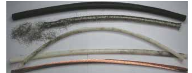
Picture 1: Damaged overall shield sample of the braid version after 250,000 movements
