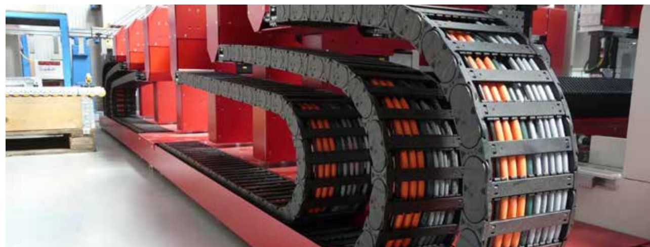
Drilling machine for wooden plates equipped with latest hybrid cable technology with Hiperface DSL
