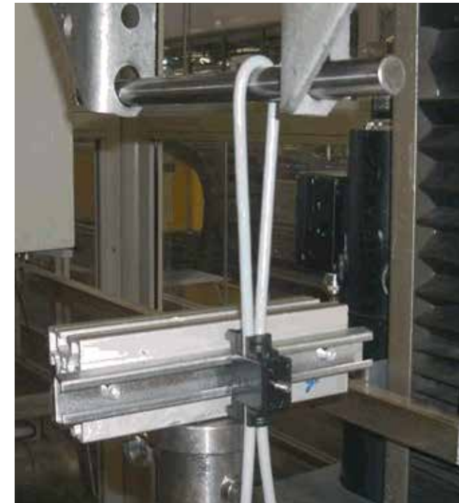
igus® tensile strength test CFX clamps with stacker saddle. Conclusion: the tensile strength of igus® chainfix clamps is three times higher when compared with conventional strain relief
