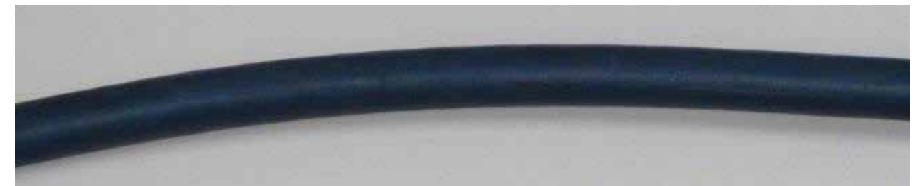
520,000 strokes without any damage, which the CF9.15.18 achieved in this test
