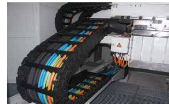
chainflex® measuring system cables in a double-spindle machining centre.
