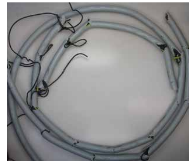
Result PUR jacket: Broken after 41,000 strokes
