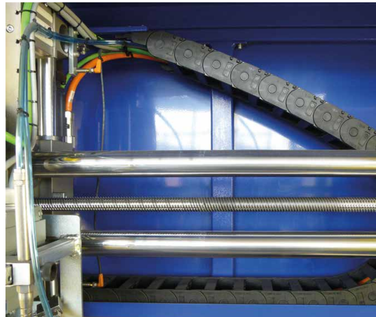
chainflex® CF270.UL.D motor cable in a system for sharpening knives
