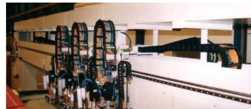
Woodworking machines with e-chains® and chainflex® cables
