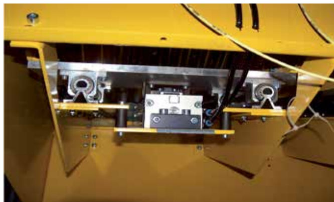
Cost-effective guide for work piece carriage in a machine tool with supported aluminum shaft.
