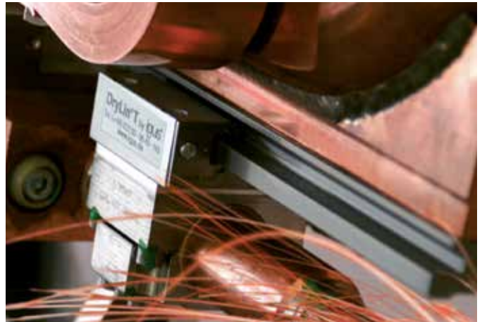
Due to the welding spatter and dust, the use of the extremely dirt-resistant drylin® T linear guide finds the balance between high service life and low costs.
