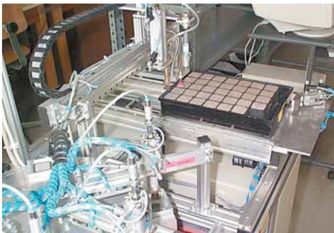
The pick-and-place unit is moved along the X-Y axis using the space-saving and cost-saving drylin® N low-profile linear guide. The drylin® T guide system is used for vertical guidance.
