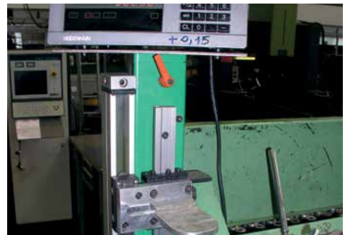
Time saving: Reduced tool changing time due to this measuring system. The gauge is guided on a drylin® T rail. This solution works also without problems in dusty environments.
