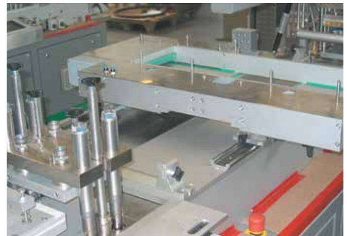
drylin® W guide rails are accredited to cleanroom-standards and therefore used in this blister machine
