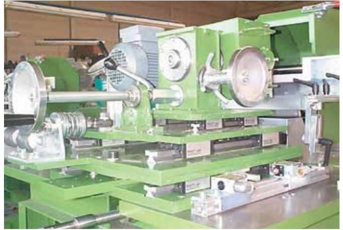
drylin® T replaced ball bearings on this grinding machine exposed to metal shavings
