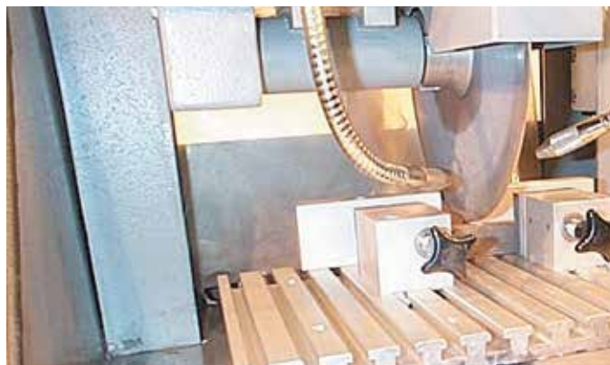
Stainless steel combined with iglide® J in cut-off grinding machine. Grinding particles and coolants, extreme conditions.
