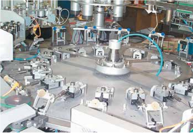
Food processing application using drylin® T in a caustic wash-down environment
