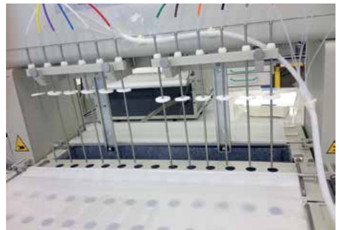
This sampling device uses drylin® linear plain bearings to remove the products precisely and smoothly.
