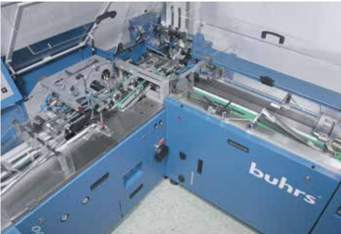
The drylin® T linear guides are used in these enveloping machines to guide an envelope suction opener that is mounted on one side.
