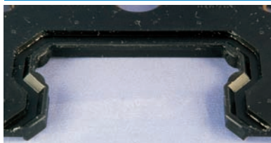
Lip has not been fractured
