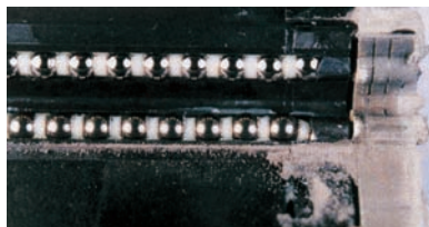
No foreign matter entering the raceway observed
