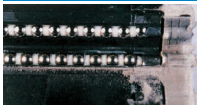
No foreign matter entering the raceway observed
